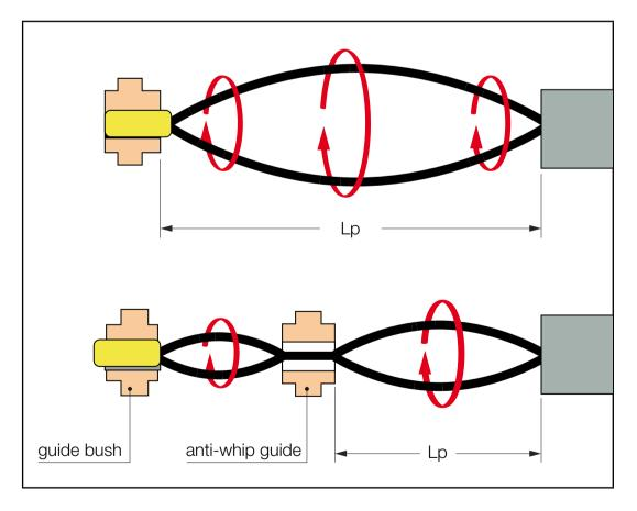
If the parameters are in the deformation zone as shown below, cutting speed amending or use of guides for support should be considered to avoid the whip phenomenon.
